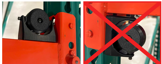
Directional sensor must be installed on horizontal surface.
